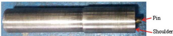
Fig. 1 FSW tool made of H13 tool steel
